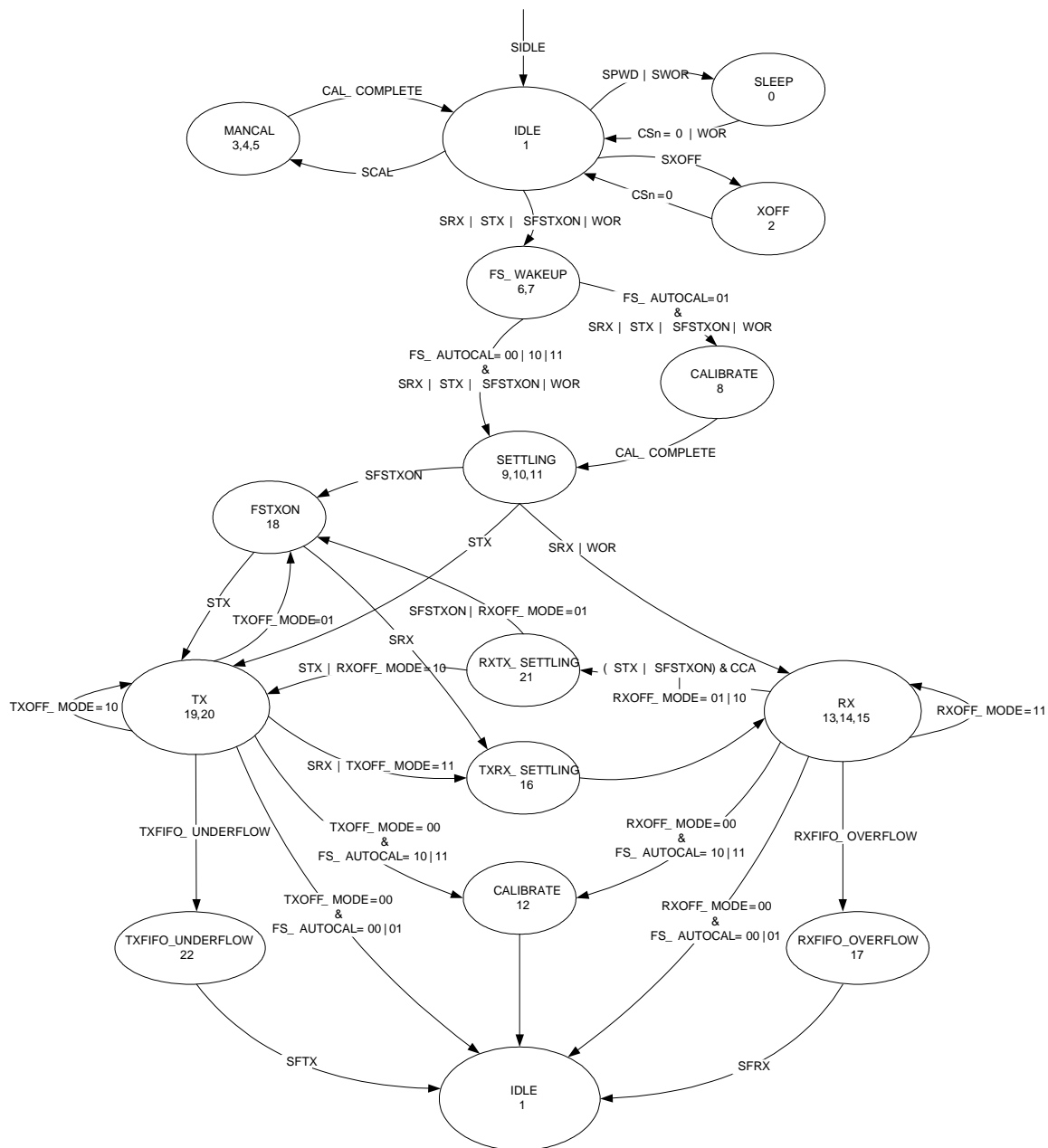
Figure 15: Complete Radio Control State Diagram
