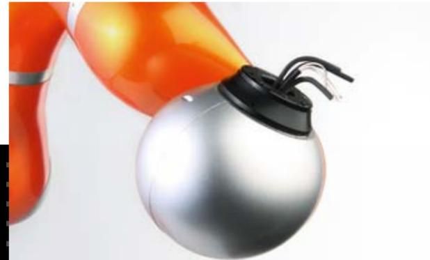
Well-rounded: the power supply right up to axis 7 is routed internally. There is no additional disruptive contour.
