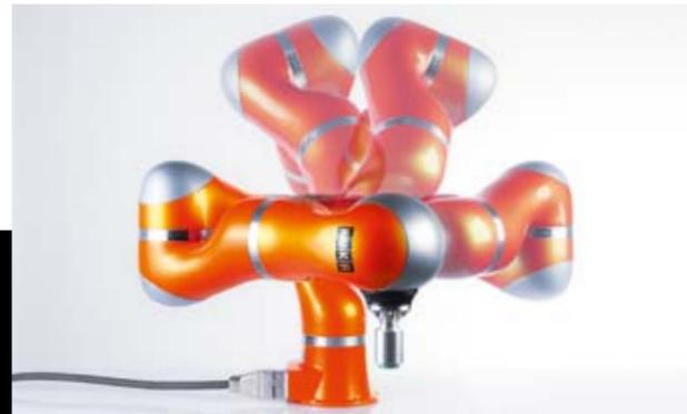
Redundancy due to the seventh axis: for a given position and orientation, a pose can be selected that is favorable for the process concerned.
