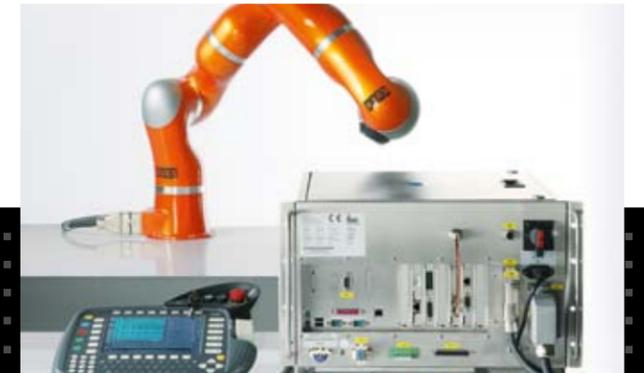
A dynamic trio: LWR 4+ with the service-proven KUKA KR C2 lr controller and the KUKA teach pendant.
